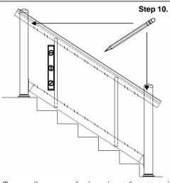
Temporarily remove aluminum insert from top rail and position uncut top rail onto pickets. Make sure that pickets are inserted into the same corresponding routs as bottom rail. Using a level, ensure that pickets are plumb. Scribe top rail as in Step 3. Now remove top rail.
