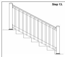
Reinstall the now cut top rail with aluminum insert onto pickets. Ensure pickets insert fully into top rail and extend all the way to aluminum insert (approximately 2 inches). Position and install top rail to posts. Refer to steps 7 & 8 to attach brackets.
