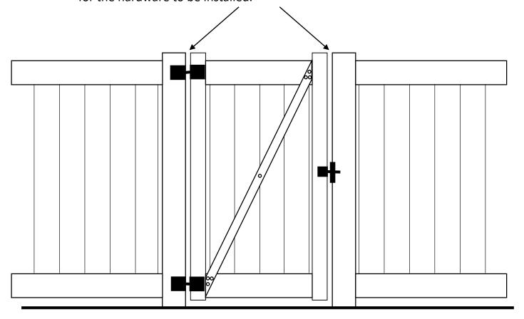
The gate should always be hung with the bottom of the cross brace on the hinge side of the opening. Its purpose is to help hold UP the weight of the free hanging side of the gate.
