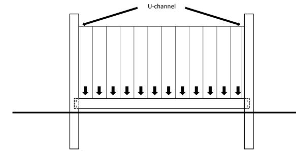
Insert your T&G pickets into the bottom rail. Make sure that the tongue from the first picket is inserted into the groove of the next picket. These pickets are meant to interlock with one another to provide stability and added wind resistance.
