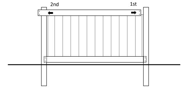
Once you have your pickets in place, lean them forward slightly to allow you to put the top rail on the top of the pickets as pictured. Once in place, slide the rail across the pickets and insert the end of the rail into the post. Do this in the same manner as the bottom rail, working towards the leading post and allowing the trailing end of the rail to clear the previous post so that it may be inserted into the rout.
